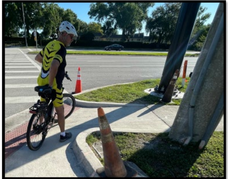
Image 14- Cyclists must turn a long distance on sidewalk curb to reach pedestrian push button.
